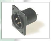
XACM / PCS 3 Pin vertical PCB mounting Male XLR with non counter sunk mounting holes for self-tap screw fixing. ACM PCS has counter sunk mounting holes for M3 screw fixing. Nickel Silver plated Brass contacts.
