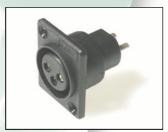
ACF 3 Pin chassis mounting Female XLR with counter sunk mounting holes for M3 screw fixing. XACF has non counter sunk mounting holes for self-tap screw fixing. Nickel Silver plated Brass contacts.
