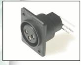
XACFR / PC 3 Pin horizontal lateral right PCB mounting Female XLR with self-tap screw fixing. Vertical PCB mounting versions ACF / PCS and XACF / PCS available. Nickel Silver plated Brass contacts. ACFR/PC (CP30016) XACFR / PC (CP30017) ACF / PCS (CP300125)
