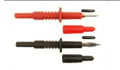
TPR/1S Spiked test probe. Unfused. Has 4mm. shrouded socket connection, so converts 4mm. shrouded plug into a test prod lead. 1KV CAT III with tip cover fitted. CAT II without.
