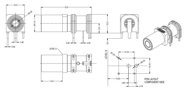
These 4mm sockets consist of two insulated, semi-circular contacts, which are connected to each other when a plug is inserted (switch function). The socket is PCB mounted.
