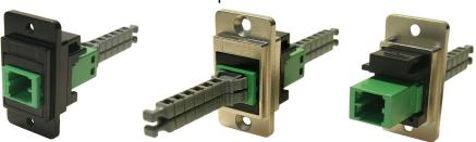
MMC is a Very Small Form Factor (VSFF) multi-fibre optical connector designed for termination of multiple single-mode and multimode fibre cables in the AI Data Centre environment. This 2 port MMC Feedthrough Adaptor will accept one or two US CONEC APC polish connectors and is supplied with two single port dust covers on the front and rear (four in total).
